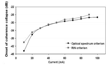
Fig. 2. Onset of CC, determined both from the optical spectrum and the RIN, of a 205- $\mu$ m- long DFB quantum-dash-based laser versus the injection current. Reprinted with permission from [12].
