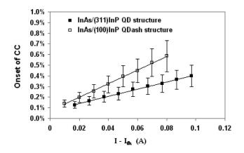
Fig. 11. Onset of CC as a function of the current difference for a 1100- $\mu$ m-long quantum-dot-based laser and for a 1200- $\mu$ m-long quantum-dash-based laser.
