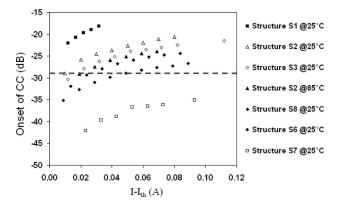
Fig. 10. Onset of CC of 600-µm-long quantum-dash-based lasers (the dashed line represents the minimum value required for isolator-free operation).
