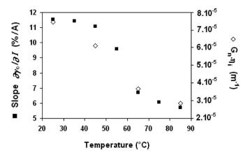
Fig. 6. Parameter  $G_n \eta_i$  and slope  $\partial \gamma_c / \partial I$  versus temperature.
