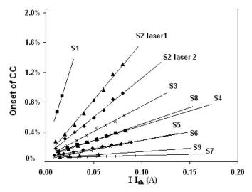
Fig. 3. Onset of CC of several 600  $\mu$ m-long Fabry–Perot quantum-dashbased lasers as a function of the current difference. Reprinted with permission from [23].
