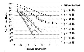
Fig. 9. BER versus received power for different feedback levels at 30 mA. Reprinted with permission from [12].
