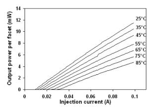
Fig. 4. Light–current characteristic of a quantum-dash-based laser as a function of the temperature.
