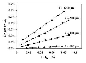
Fig. 7. Measured onset of CC of quantum-dash-based lasers of the same structure and fabrication process as a function of the cavity length.
