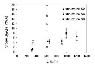
Fig. 8. Measured slopes of the onset of CC with injection current as a function of the cavity length for three distinct structures.
