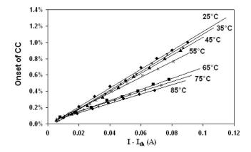
Fig. 5. Measured onset of CC of a quantum-dash-based laser as a function of the current difference and temperature.
