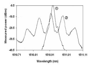
Fig. 1. Optical spectrum: (1) without optical feedback; (2) with optical feedback and onset of CC Reprinted with permission from [12].
