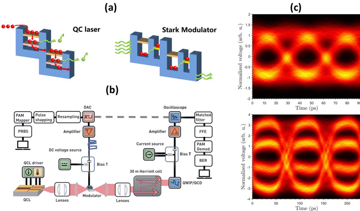
Fig. 1: (a) Building blocks of the unipolar quantum optoelectronics system; (b) Schematic of the full transmission setup including a QCL and the Stark modulator. The signal goes through the Herriott cell before being collected on a high-speed detector (QWIP/QCD) and recorded with a fast oscilloscope; (c) Recorded eye diagrams at 30 Gbits/s (OOK) and 24 Gbits/s (PAM-4) after 31-meter propagation distance when taking into account both pre- and post-processing.
