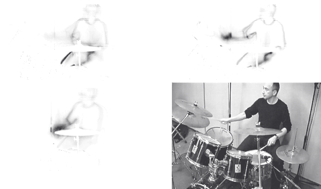
Fig. 2. Examples of computed masks: gesture for bass drum (the pedal is kicked by the right foot), gesture for the cymbal at the right of the drummer, gesture for the low tom at the right of the drummer, and reference image.
