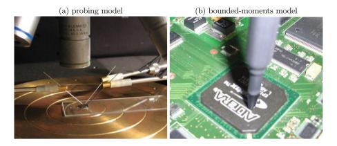
**Fig. 1.** Settings for side-channel analysis. In the probing model (a), a few bits (here, d=3) are measured with dedicated probes. In the bounded moments model (b), the attacker measures an integrated quantity of several bits.
