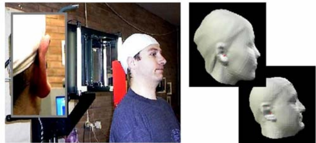
Fig. 1. Laser scan acquisitions of 41 people. At right, two renderings of the triangular mesh models in VRML format.
