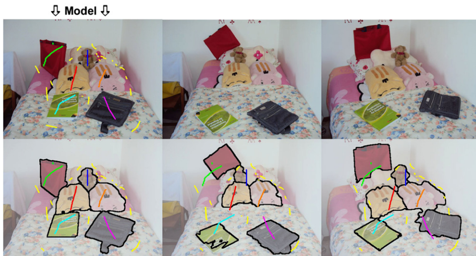
Fig. 29. Example with large variability of the color information. Similarly to the former figure, the scribbles were drawn over the left image, chosen as the model. Each segmentation was obtained by matching the model graph with each input graph corresponding to each image.
