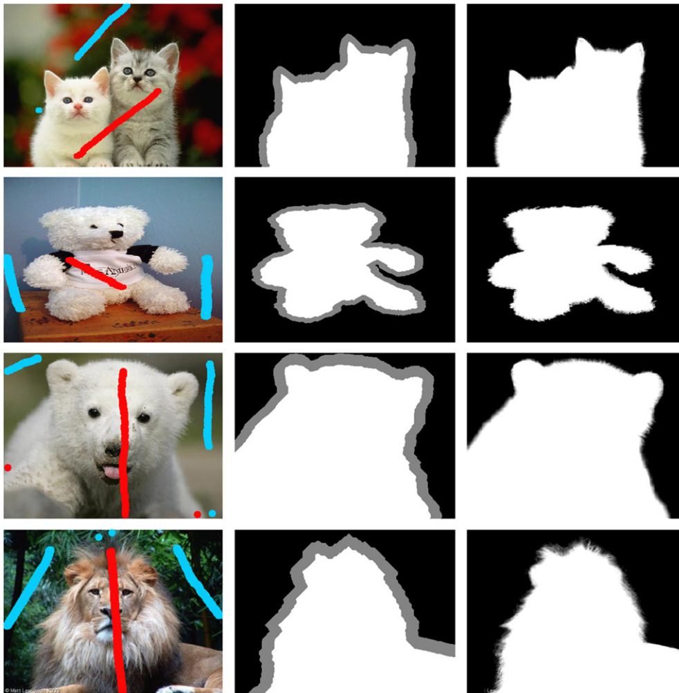
Fig. 21. Input images from Bai and Sapiro [4,5]. Left column: original images with scribbles. Middle column: automatically computed trimaps by DG+P1+P2. Right column: alpha mattes computed by Robust Matting [35] using the trimaps from the middle column.
