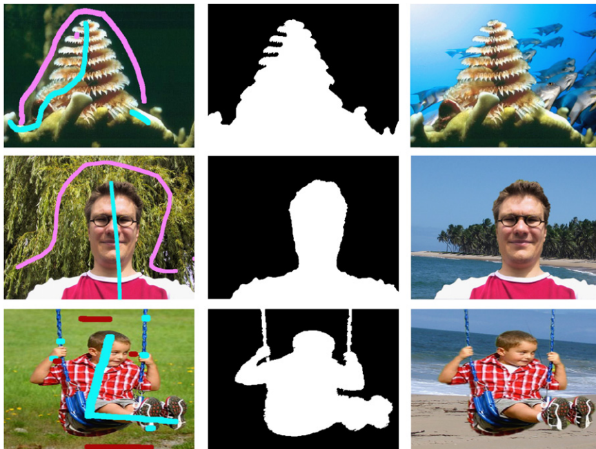
Fig. 14. Examples of background replacement using images from different databases: Berkeley [22], GrabCut [28], and Bai and Sapiro [3,5], respectively. Left column: original images with scribbles. Middle column: labels computed by the proposed approach (DG+P1+P2). Right column: compositions using new backgrounds.
